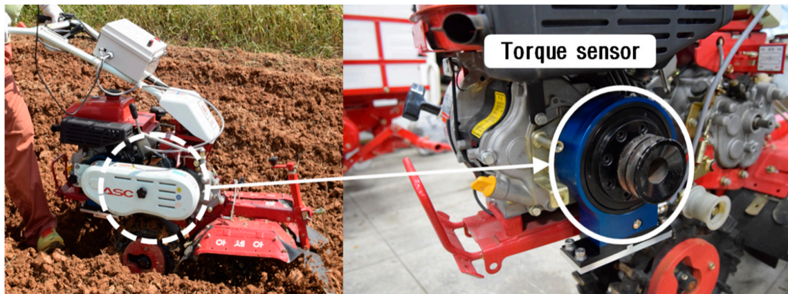
Figure 2. Torque measurement system for the cultivator.
